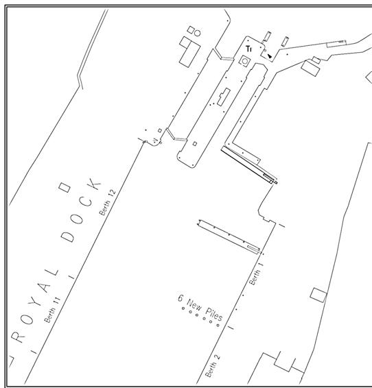
6 piles will be installed approximately 75m South of the current pontoon on berth number 1. The outermost pile will be positioned 45m into the Dock and will be lit with two fixed red navigation lights positioned vertically.
